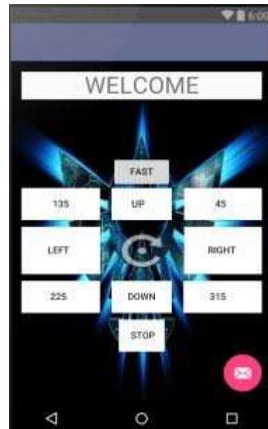
Fig 6: Android app for the operation of Wheelchair.
